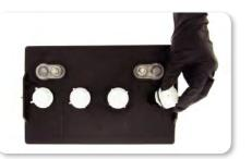
Remove the vent cap from the proper cell.
